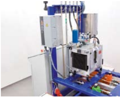
Mixing head hydraulics, gear type volume sensors and external frequency converters
