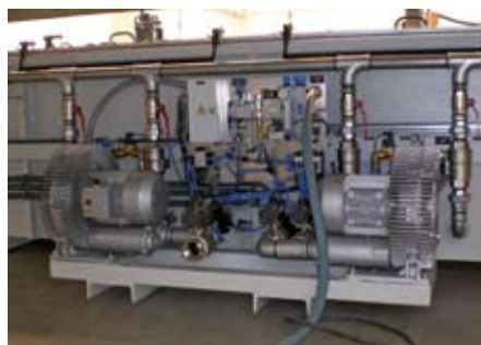
Pre-blowing and vacuum distribution
