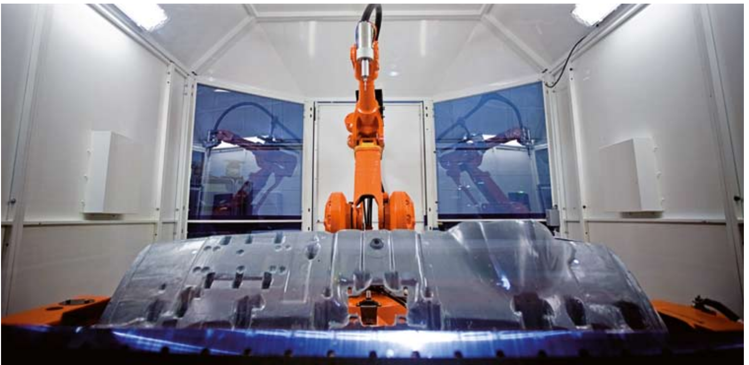
FlexTrim router cell with one robot and prototype fixture
