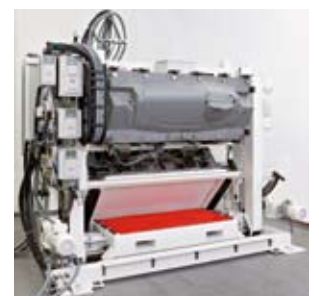
Pivoting of the upper carrier by 180° enables simultaneous handling on both sides
