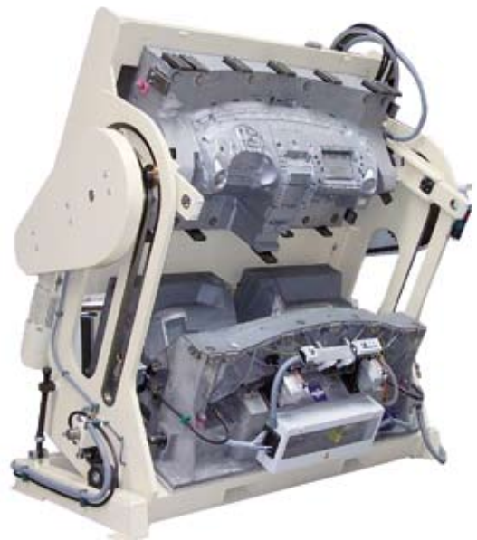
Basic version with manual adjustment of foam pour direction
