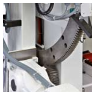
Foam position: pivot drive via rack and pinion stern segments, seamlessly adjustable from -35° to +35°
