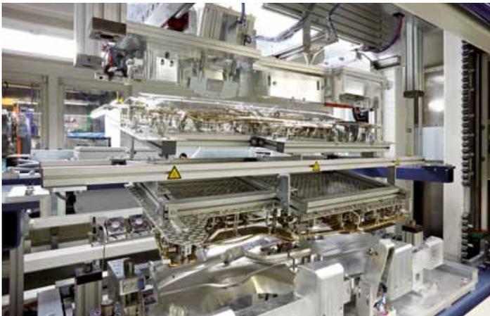
Complex infrared (IP) tool with standard emitters, contour emitters and shadow plates.
