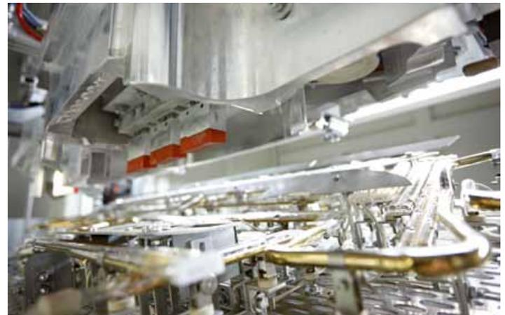
Component fixture with independently powered 3D holding-down system
