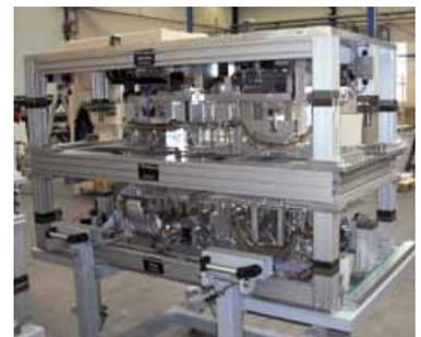
Easy tool change by means of sandwich design
