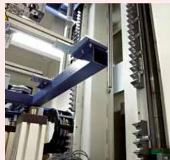
Lifting gear with the roller pinion system (RPS), drive via servo geared motors with absolute encoder.
