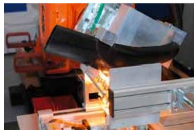
For infrared joining, different types of IR emitters can be used. Depending on the project requirements, quartz glass bulb emitters or metal foil emitters can be used. FRIMO offers tailor-made solutions for both systems.
