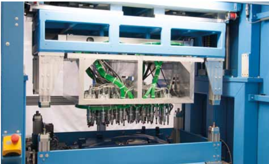
Complex tool for heat staking
