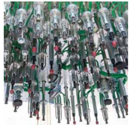
Complex tool for heat staking
