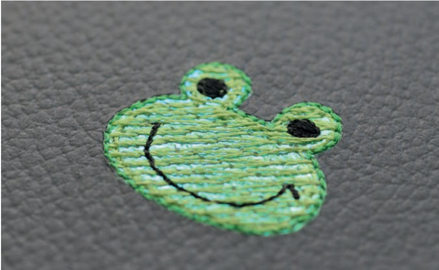
Fig. 3. IMG enables the attachment of individual symbols on the surface
