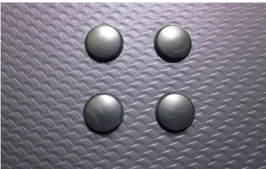
Fig. 4. So called pads integrated with the IMG process
