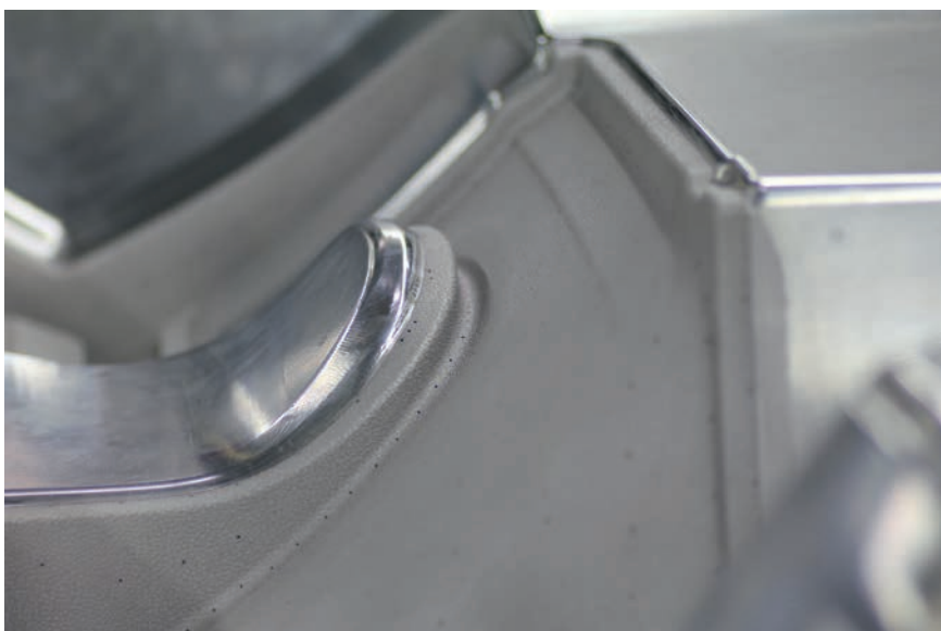
Fig. 2. Grained shell mold for the in-mold graining (IMG) process
